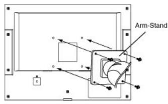
4 Mounting Screws (enclosed): M4 x 12 mm
